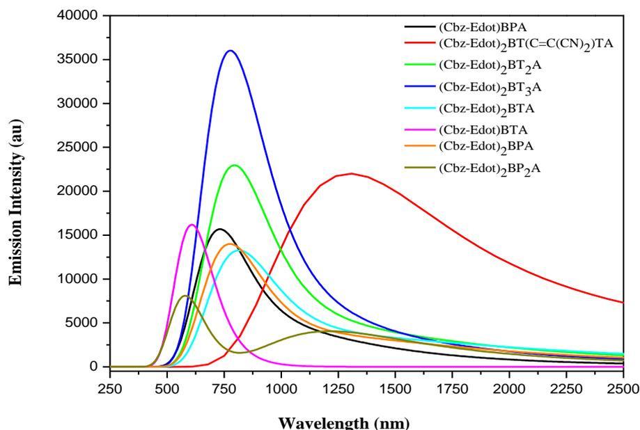
**Figure 5 :** Simulated emission spectra of the studied compounds calculated by TD/DFT/B3LYP level using CIS/3-21G\* optimized geometries.
