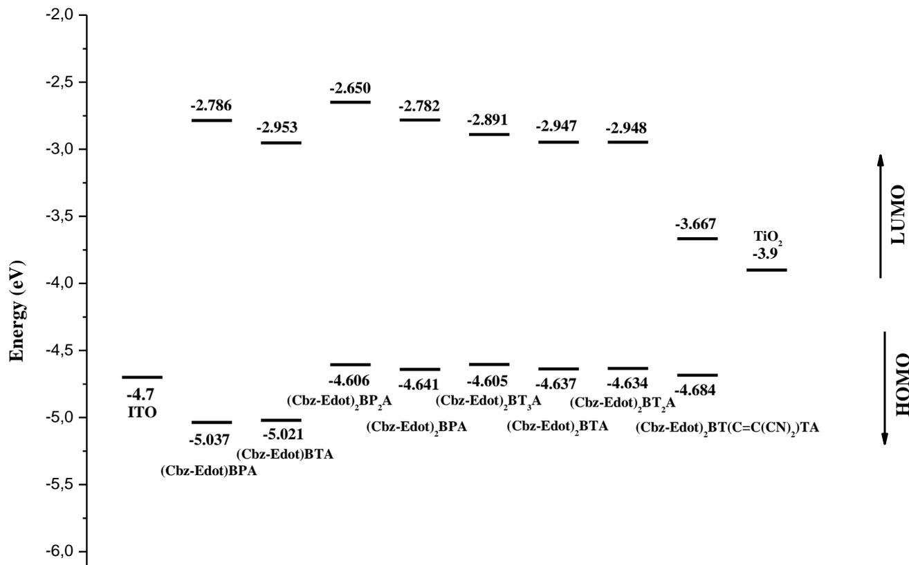
**Figure 2 :** Sketch of B3LYP/6-31 G (d,p) calculated energies of the HOMO and LUMO level of the studied molecules.
